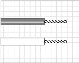
Speakers and electronics terminals have corresponding (+) and (-) terminals. It is important to connect both speakers identically: (+) on the speaker to (+) on the
